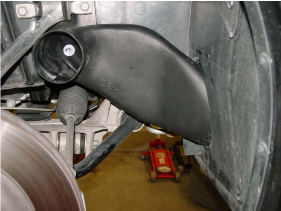
Screw location to mount the brake duct. Place the screw/washer through brake duct outlet after trial fit and drilling pilotheole. (as pictured above)
