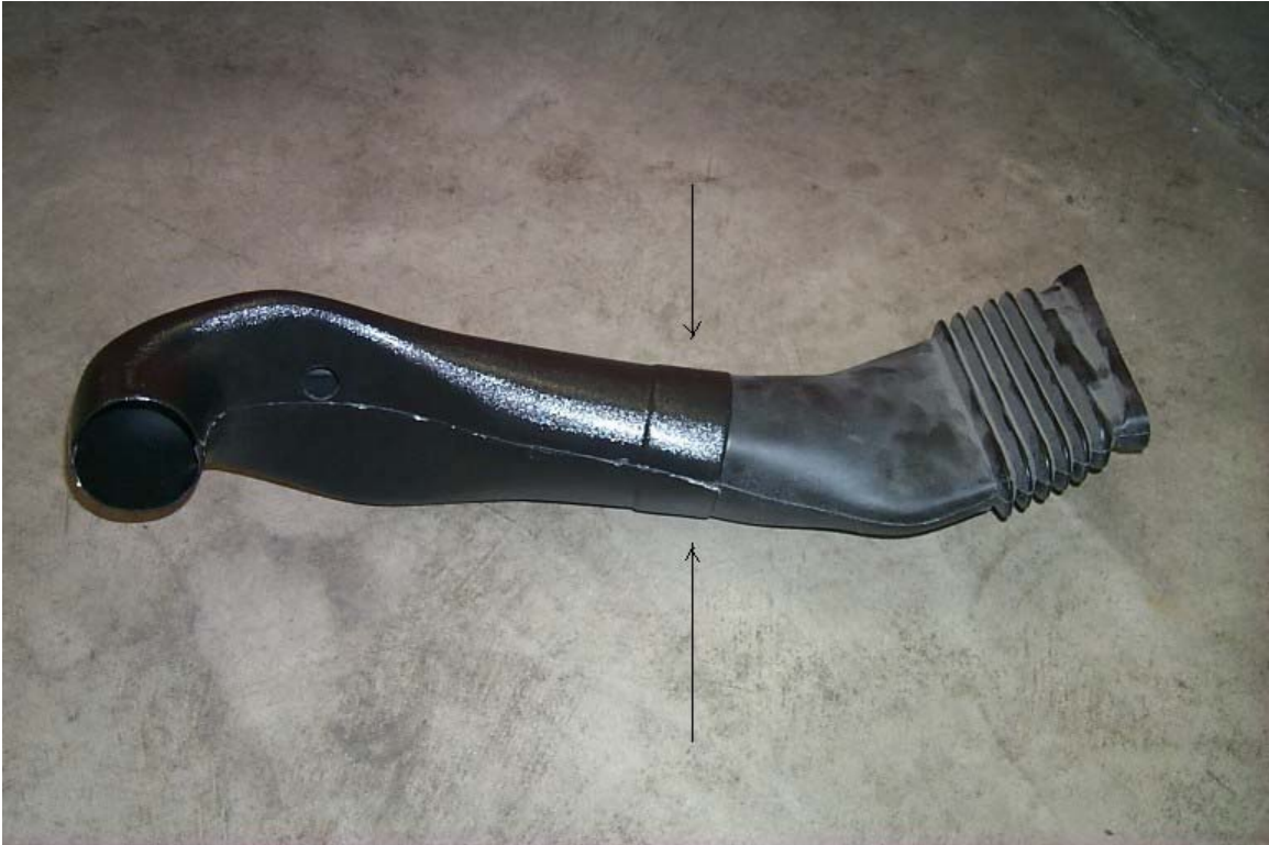
Place a screw to fix the ducts after trial fit.
